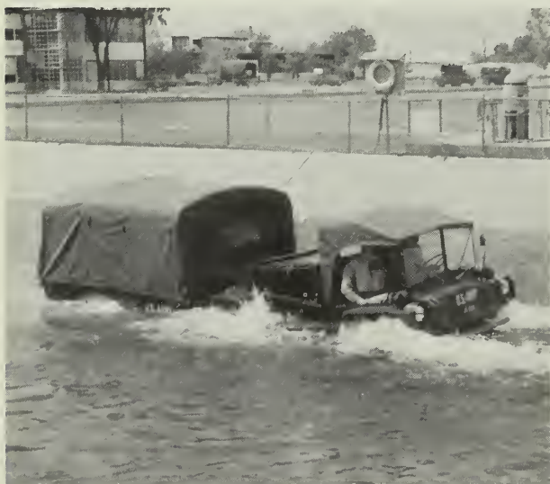
ARMY is testing XM 561 jointed cargo carrier, which goes equally well in the water (left) or over roughest terrain.
